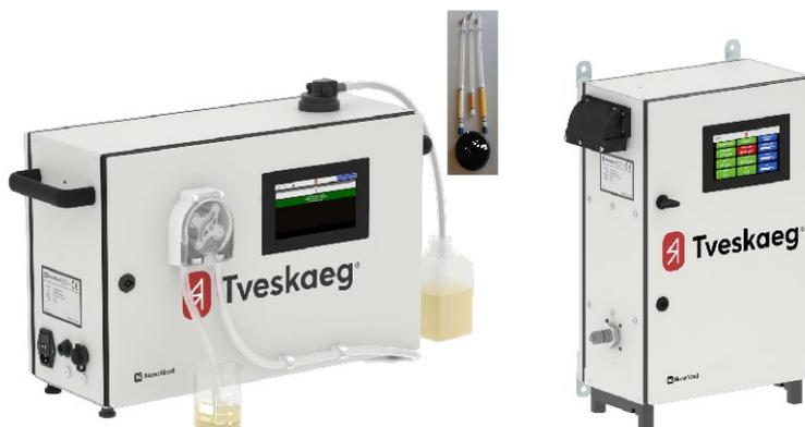
Figure 1. Two variants of the NanoNord TVESKAEG™ NMR sensor, based on a 1.5 Tesla magnet and advanced radio-frequency technology. A BENCHTOP instrument (left panel) with options for sample stick (shown in insert) or peristaltic pump (on the front of the spectrometer) sample insertion. A FLOW instrument (right panel) to use for inline continuous measurement in a production line.
